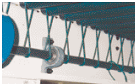
Live rollers - power transmission
